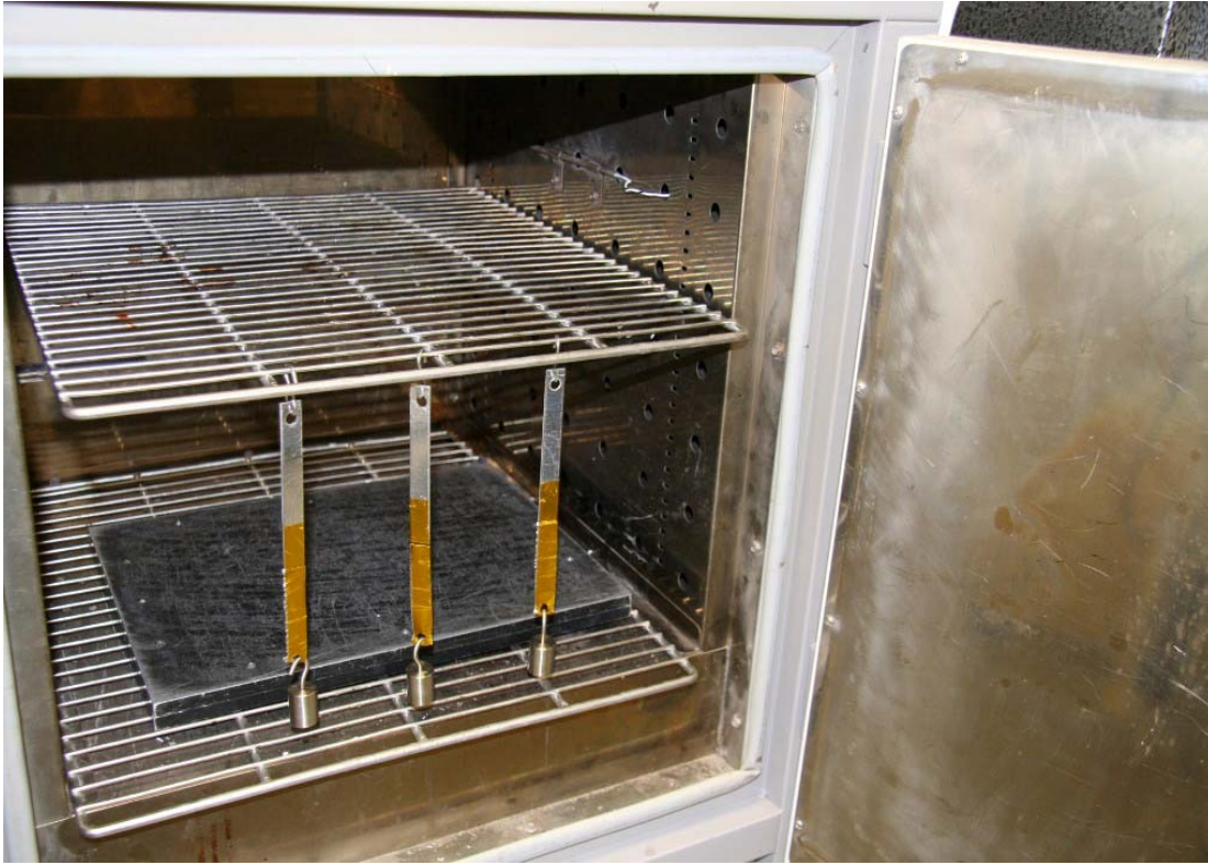
Figure 3: Static Shear test; PSA coated onto Kapton and bonded to aluminum panels.
